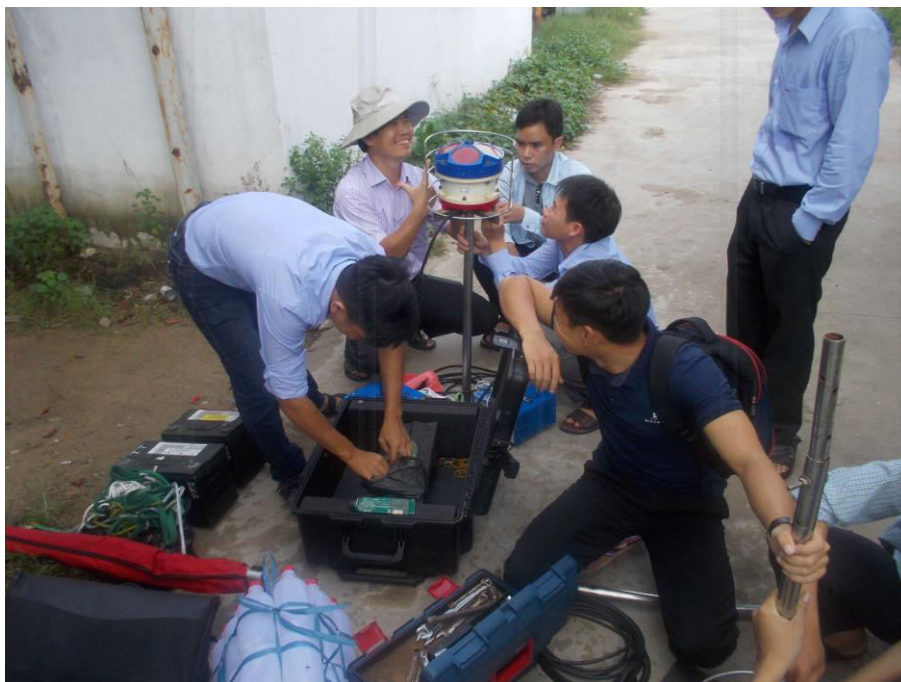
Figure 1: Field experiment set-up: 600 kHz ADCP (RDI) with batteries, sampling bottles
